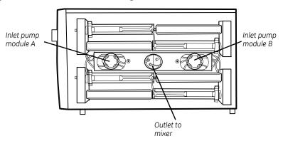
In ÄKTAfplc, the inlet and outlet tubing are installed at the factory.
