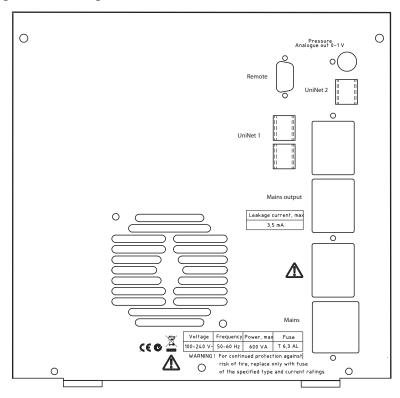
The sockets for electrical signals are located on the rear panel.
