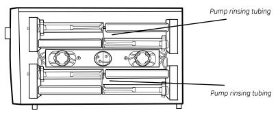
The rinsing tubing for the piston seals is installed at the factory and filled with 20% ethanol. Check that the rinsing solution is present behind the pistons and that the rinsing tubing is connected and undamaged. Always use 20% ethanol as rinsing solution. Change rinsing solution at least every month.
