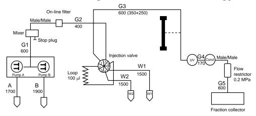
The G3 capillary is mounted at the factory as a column bypass. It is used initially during the installation test. When the test is complete and a column is to be fitted, the G3 capillary can be cut and used to connect the column. The figures state the length in millimetres of the prefabricated capillaries.
