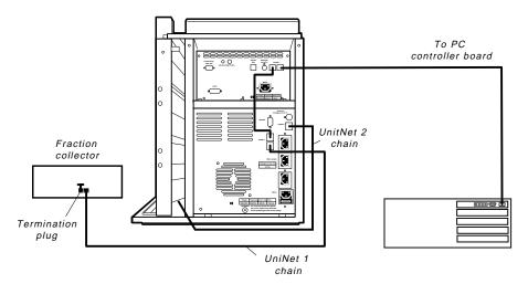
The UniNet 1 data communication chain is routed from the computer via UPC-900 and P-920 to the fraction collector. The chain is terminated at the fraction collector with a termination plug.
