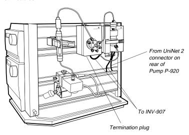
The UniNet 2 data communication chain, which controls the valve(s) and the mixer comes from the rear of Pump P-920. The chain is terminated at the injection valve with a termination plug.
