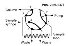
**Note:** No more than half (50%) a loop volume of sample should be loaded into the loop.
