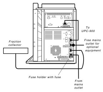
Only one mains input is required for the complete system. The supply voltage for the components in the system and the fraction collector is distributed from the base of the system. The mains input fuse holder is located below the mains input.
