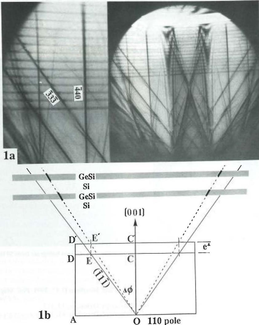
Fig.1 a [110] LACBED pattern of the  $\text{Ge}_x\text{Si}_{1-x}/\text{Si}$  SLS showing the shift of  $\bar{3}\bar{3}\bar{3}$  lines in GeSi layers by the strain  $e^\perp$  along [001].
