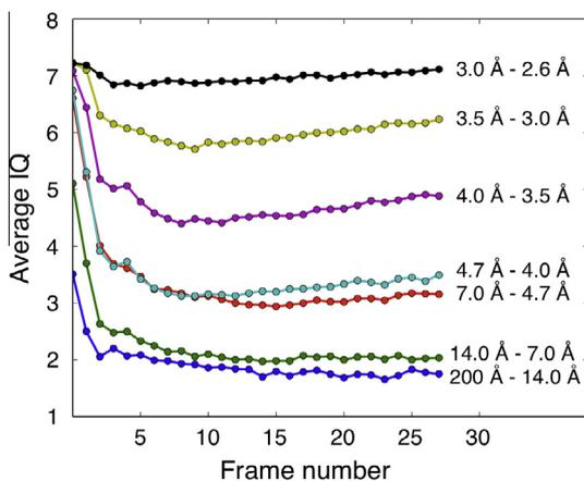
**Fig. 3.** Analysis of the effect of increasing electron dose on the average IQ values of diffraction spots in resolution bins. The average IQ values were calculated for the indicated resolution ranges and plotted against the cumulative frame number.
