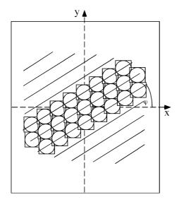
Fig. 5. Determination of tilt axis. Power spectra are calculated for each tile along the eleven parallel lines (tiles are only indicated for the three central lines). The angle  $\varphi$  is searched in 2° steps to find the direction in which the variance between the power spectra is minimized.
