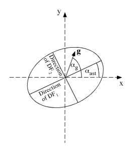
Fig. 3. Definitions for the CTF parameters DF<sub>1</sub>, DF<sub>2</sub>, and  $\alpha_{ast}$ . The angle  $\alpha_g$  of the scattering vector  $\mathbf{g} = \mathbf{k}' - \mathbf{k}$  ( $\mathbf{k}$ , wave vector of the incident wave;  $\mathbf{k}'$ , wave vector of the scattered wave) is used in Eq. (6), indicating the point where the CTF is evaluated.
