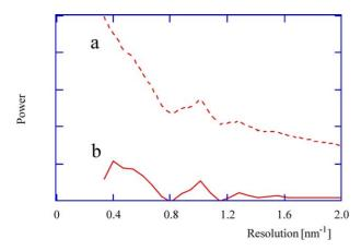
Fig. 2. Background subtraction (a) shows a plot of a radial average of the power spectrum obtained for image b3730 (see Table 1). Before fitting defocus values, the smooth background has to be subtracted. The radial average of the background-subtracted power spectrum is shown in (b).
