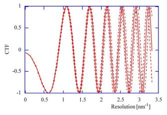
Fig. 7. Error in the measured defocus value. The CTF is plotted for different defocus values. The solid line shows the CTF for an underfocus of 500 nm, and the two dotted lines show CTF plots for 490 and 510 nm underfocus. Seven percent amplitude contrast was included in these plots, and a microscope running at 200 kV and a spherical aberration coefficient of 2 mm were assumed.
