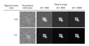
Figure 3 Test patterns with  $64 \times 64$  pixels and signal-to-noise ratios of 1/25 and 1/4 and data-set averages after 30 cycles of translational alignment for data sets containing M = 1000, 5000 and  $10\,000$  images.
