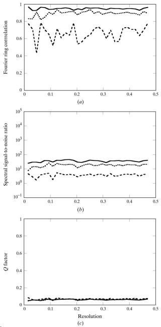
**Figure 1** (a) FRC, (b) SSNR and (c) Q factor in resolution zones for aligned data sets with images containing only normally distributed noise. The data sets contained M = 1000 (dashed lines), 5000 (dotted lines) and 10 000 images (unbroken lines). The noise in the plots is highest for the smallest data set. All plots show approximately constant values across the spectrum. The resolution is given in units of pixel<sup>-1</sup>.
